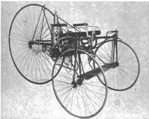
8. New Englander George Long built this unusual steam tricycle in 1879. It seated two passengers side-by-side (usually needed two to run it) and featured a five-foot driving wheel in the rear, three-foot wheels in front. A two-pulley arrangement from engine to wheel gave Long's machine a two-speed "transmission."
