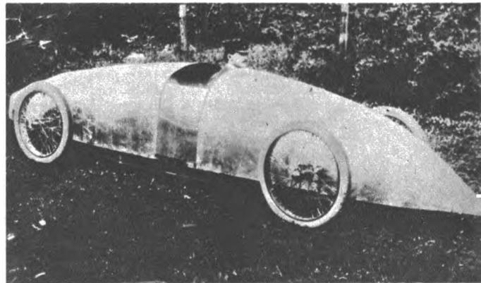
9. The "Woggle Bug" was the ultimate in the development of the steam car. This one won a batch of speed trophies in 1905 and a similar model was the first motor car to reach the amazing speed of almost 120 mph when it did two miles under a minute in 1908. However, the rise of the gas-driven car was slowly eliminating steam cars.
