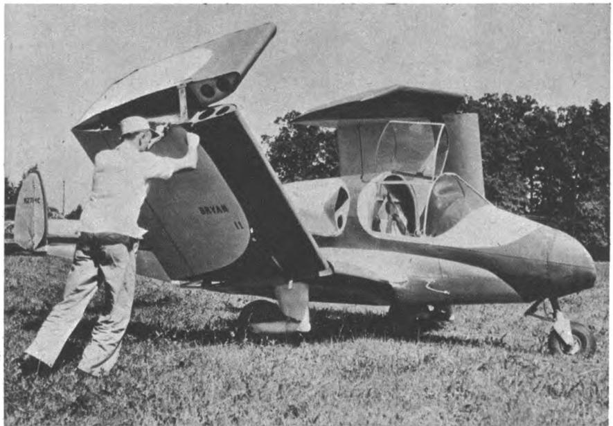
Conversion of car to plane takes only 10 minutes. Lowered wings have span of 22 feet. Craft needs minimal area for take-off.
