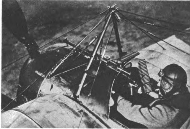
This rare photo shows how machine gun first fired through prop.
