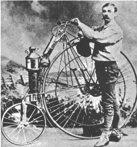
5. Mustachioed Copeland with his 1884 steam bicycle. Using the high-wheeled bicycle of the era, he mounted a copper-and-brass boiler on the front bar of the cycle and ran pulleys to the rear wheel for power. Water tank held enough water for 30 minutes run. Cylinder had 1/16-inch bore with a three-inch power stroke.
