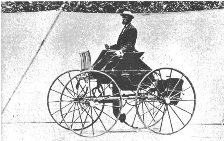
2. Sylvester H. Roper was one of the most prolific steam vehicle builders. Here he sternly grips the throttle of one of his later inventions, a steam-driven, four-wheeled wagon of about 1870, now referred to as the Roper Steamer. Roper, a great experimenter with steam motorcycles, delighted in racing his steam-driven machines (both wagons and cycles) against horses at county fairs.
