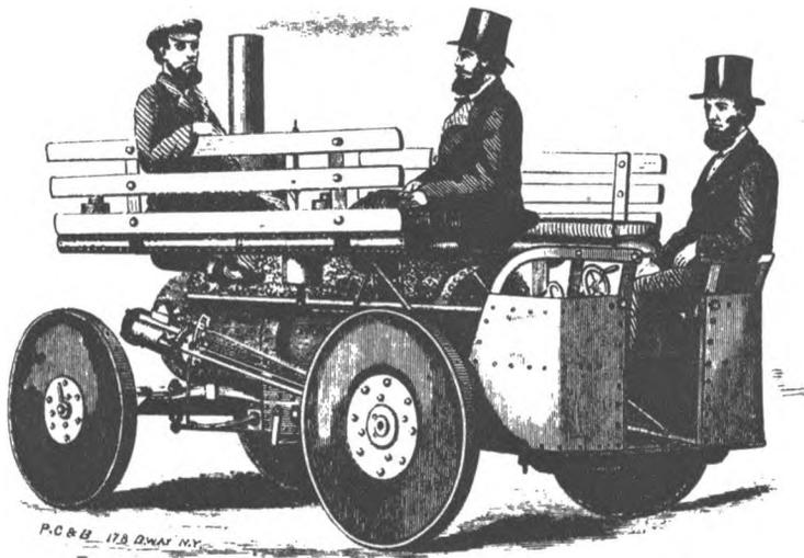
7. One of the earliest—and largest—of the steam vehicles was Richard Dudgeon's 1867 10-passenger steam "wagon." The New York inventor's machine ran on four wooden wheels with the rear ones connected to steam cylinders. The front axle was mounted on a pivot for road steering.
