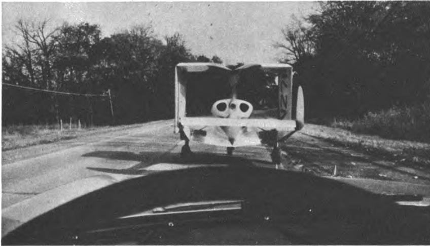
On open road, 17-ft. vehicle will do 60 mph, powered by push-propeller. Wings fold up, lock on top of chassis.
